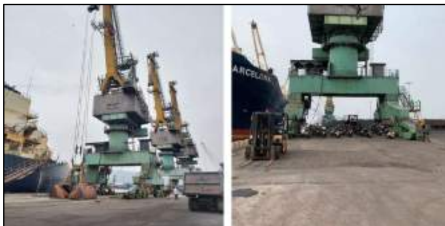
Figure 3-6 : 15T Capacity RMQC at Berth EQ-06
