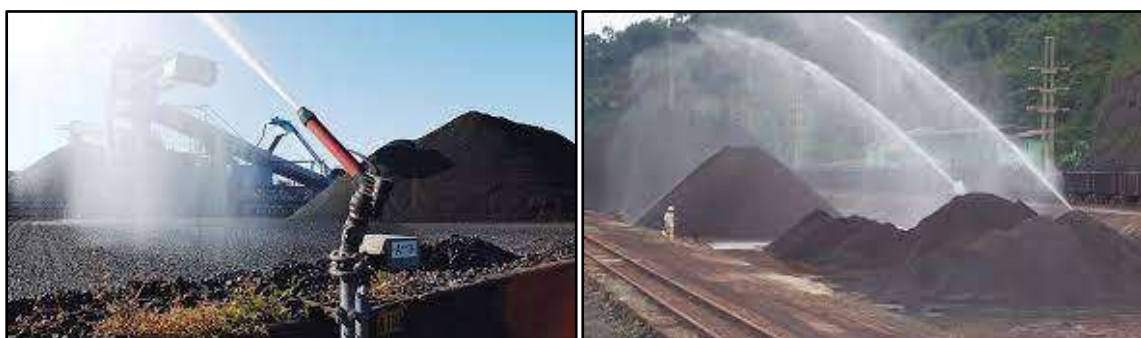
Figure 6-4 : Dust Suppression System using water sprinklers
